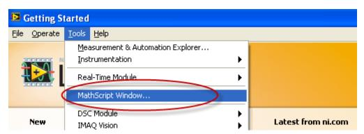
The "LabVIEW MathScript Window" is an interactive interface in which you can enter .m file script commands and see immediate results, variables and commands history. The window includes a command-line interface where you can enter commands one-by-one for quick calculations, script debugging or learning. Alternatively, you can enter and execute groups of commands through a script editor window.
