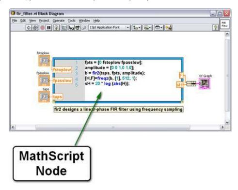
You can define named inputs and outputs on the MathScript Node border to specify the data to transfer between the graphical LabVIEW environment and the textual MathScript code.
